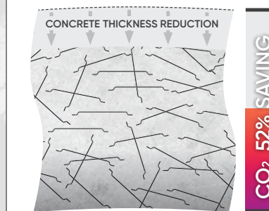
Steel fibre reinforced sprayed concrete
